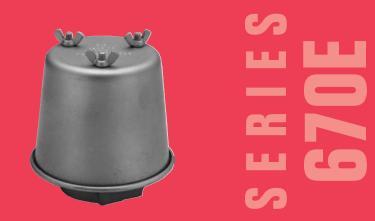
Automatic Condensate Drainage. Vertically mounted, circular plate-type flame arrester is employed for self-drainage of condensate. This prevents accumulation of condensate subject to freezing and consequent clogging of the arrester under low temperature conditions.
